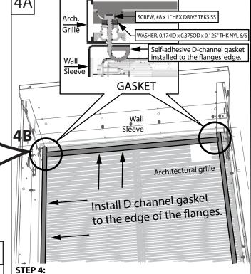
Apply self-adhesive D-Channel gasket strips (W290-0256, included with Condo Pack cabinet to inside surface of sleeve front flanges. Make sure that gasket is lined up with the EDGES of the wall sleeve flanges (detail 4A).
