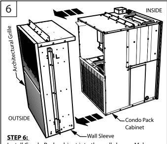
Install Condo Pack cabinet into the wall sleeve. Make sure the gaskets attached to the sleeve are not damaged. Make sure that the cabinet seats tight against the gasketing previously installed on the wall sleeve. Refer to Wall Sleeve instructions for squaring braces removal.
