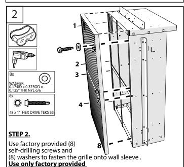
plastic washer with screws. If not used, the screws will
